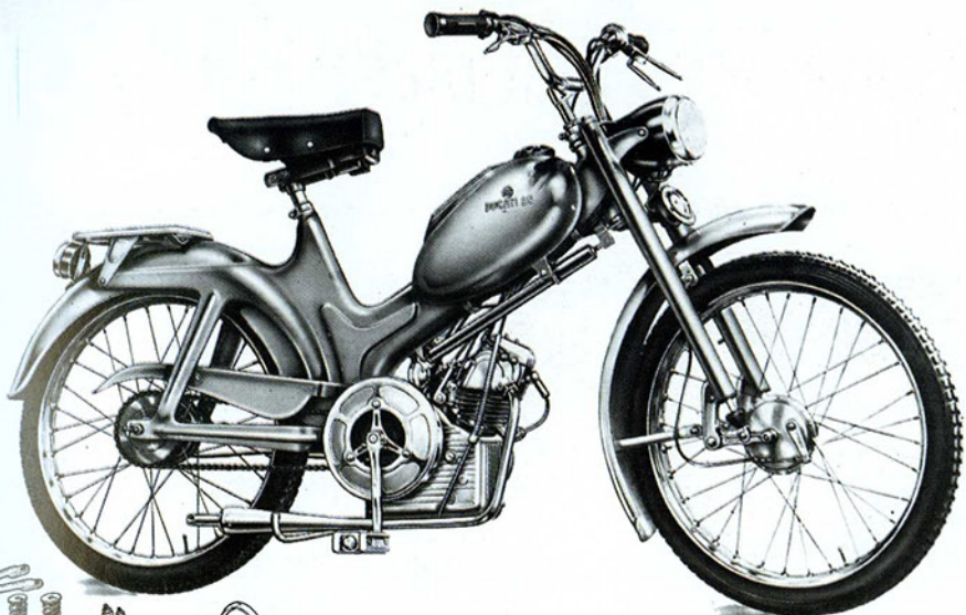
ABOVE, THE 55R OF 1954 HAD A TWO-SPEED GEARBOX WITH HANDLEBAR CHANGER AND LINK FRONT FORKS. THERE WAS NO REAR SUSPENSION BUT SUSPENSION WAS AN OPTIONAL EXTRA. THE ENGINE WAS AN M55, THE LAST VERSION OF THE FIRST CUCCIOLLO TYPE.
