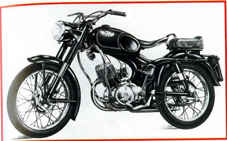
ABOVE, THE 98 T2 PRESENTED IN 1953 WAS THE MOST LUXURIOUS VERSION OF THE FIRST TYPE 98. TRIM INCLUDED LIGHT ALLOY WHEELS, CRASH BARS EITHER SIDE OF THE ENGINE, A SPRUNG SEAT AND WIDE OPEN HANDELBARS. BELOW, A 98 SS WITH THE CHARACTERISTIC SMALL FAIRING AND OIL COOLER MOUNTED TO THE FRONT OF SUMP. THIS BIKE REALLY WAS DESIGNED TO GO. EQUIPMENT INCLUDED A 20 MM CARBURETTOR, A 10:1 COMPRESSION RATIO AND A TOP SPEED OF OVER 90 KPH.
