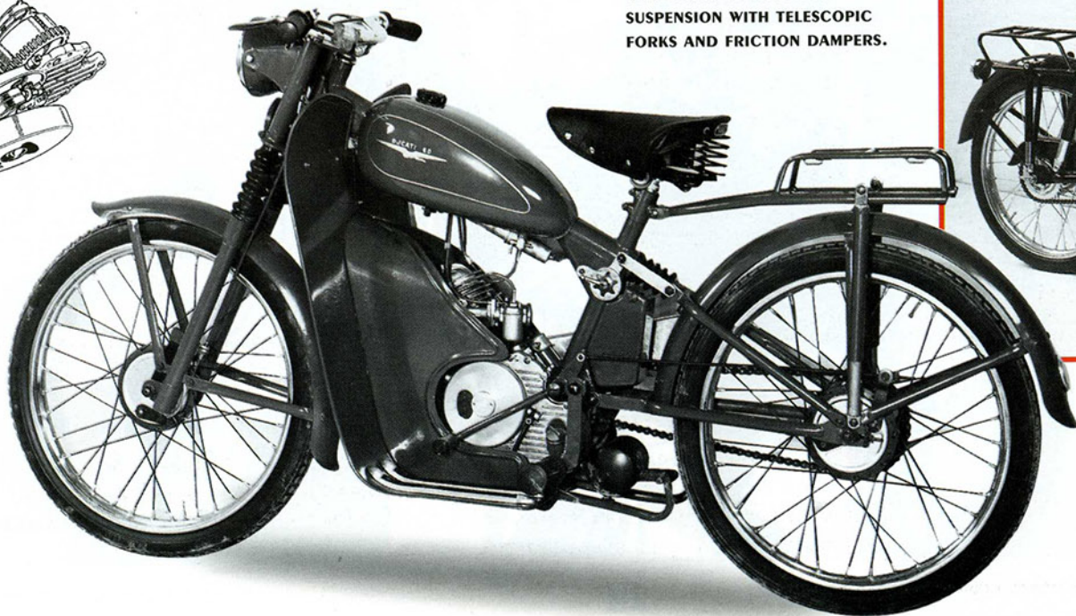
ABOVE, THE 55R OF 1954 HAD A TWO-SPEED GEARBOX WITH HANDLEBAR CHANGER AND LINK FRONT FORKS. THERE WAS NO REAR SUSPENSION BUT SUSPENSION WAS AN OPTIONAL EXTRA. THE ENGINE WAS AN M55, THE LAST VERSION OF THE FIRST CUCCIOLLO TYPE.
